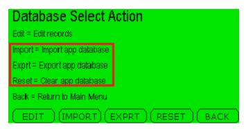
Listed in the image above are three choices for Importing (F2), Exporting (F3) or Resetting (F4) the database on your 2060. It is recommended that you export a copy of your database after making changes as this can protect data in the case of mistakes or damage to the indicator.
