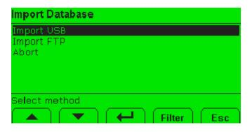
Highlight Import USB -> Press Enter -> If a USB memory device with a Database file loaded is plugged into the indicator, the screen will read, "Busy" -> When finished, the screen will return to Database Select Action Screen -> ESC to go back to home screen.
